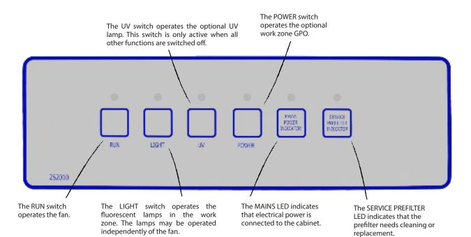
PCR Series cabinets are fitted with a low-voltage, touch-control panel to operate standard cabinet functions a general purpose power outlet (GPO) and ultraviolet (UV) lamp.
