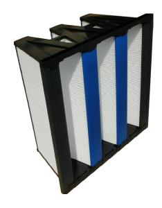
The new Nano V brings to the market an exciting change to the air filtration market. Formed through a mechanical process that integrates very fine fibre material in a manner where both coarse and fine fibers create a three dimensional structure. The coarse fibre provides the strength support and protection to the fine fibre material and through modeling we can adjust the gradient to deliver a consistent efficiency across the entire filter media.
